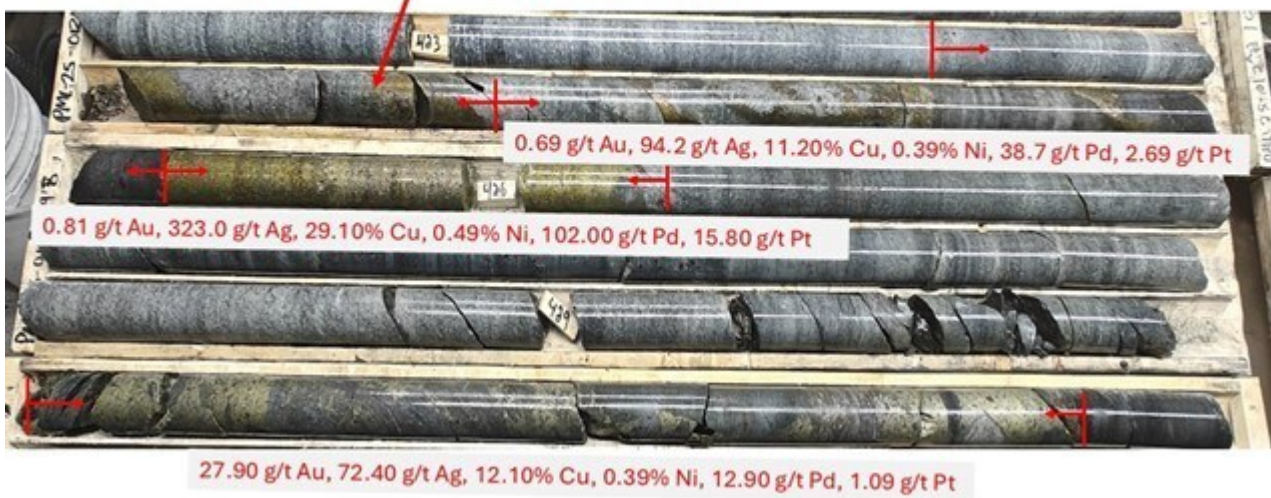
Figure 2: Core photo of high-grade mineralization in drill hole PML-25-012a with selected assay intervals.
