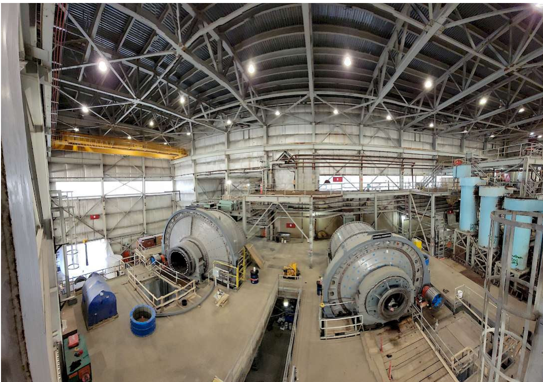
Figure 1 – Interior of mill building showing SAG (left) and Ball (right) mills installed
