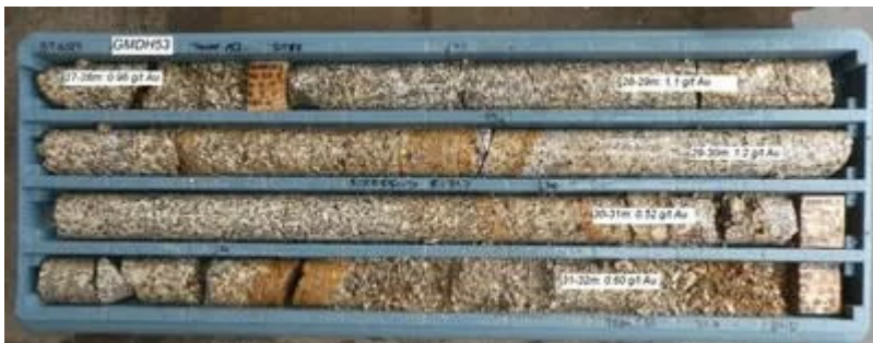
Figure 1: GMDH53 27-32m interval example of mineralised granitic drill core (CNW Group/Fosterville South Exploration Ltd.)
