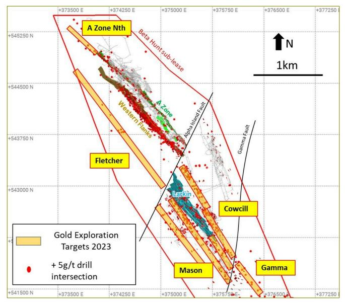
Beta Hunt plan Highlighting Mineralized zones targeted as part of 2023 exploration Drill Plan. Mineralized zones defined by +5 g/t Au drill intersections. (CNW Group/Karora Resources Inc.)
