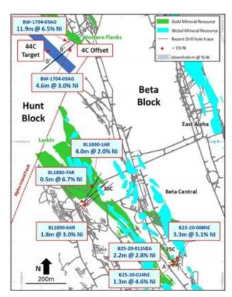
Beta Hunt plan view highlighting + 1% nickel results for the February to August 2022 period and location of 4C Offset and 44C Ni Target.
