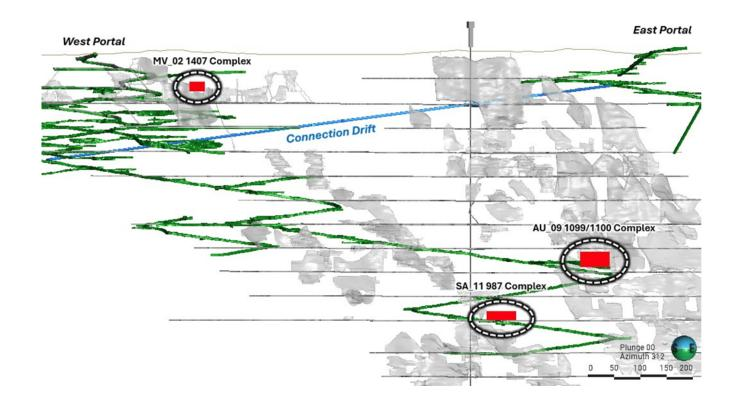
FIGURE 1: Long section showing part of the Madsen Mine deposit with bulk sample areas highlighted. Modern workings (post 2019) shown in green; Connection Drift in blue.
